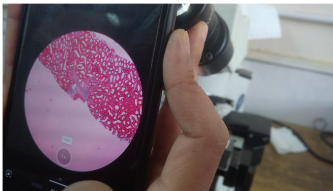
FIG 2. Images being captured by Morrison's technique without the use of an adaptor
