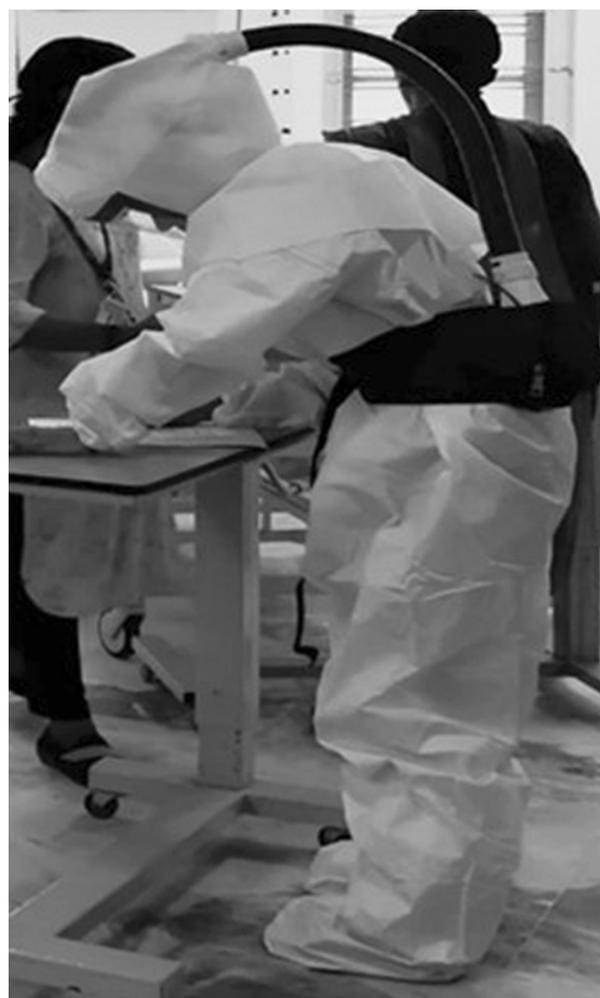
FIG 1. Low-cost powered air-purifying respirator (PAPR)
